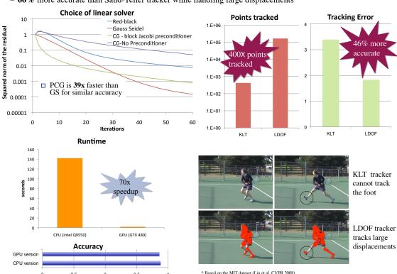
\*\* Based on particle trajectories from http://rysn.csail.mit.edu/py/data/py/ (Sand and Teller LICV 2008)
